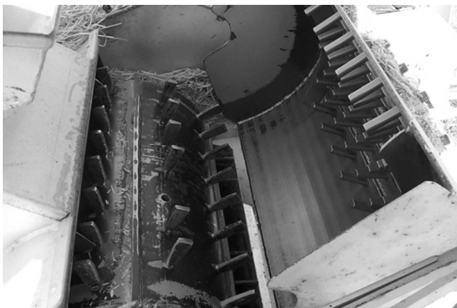
Fig. 5. Cylinder and concave tines of the tined-cylinder thresher, visible through the open cover.
